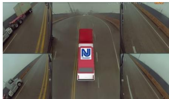
(New Jersey buses equipped with 3D SVM.)
